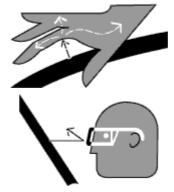
• Check for leaks by passing a piece of cardboard or wood over the suspected area.
