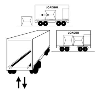
• Use a sliding bed while loading and unloading small trucks to avoid overreaching and carrying in an awkward position.
