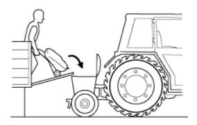
• Use ramps to avoid lifting and dragging over edges.
